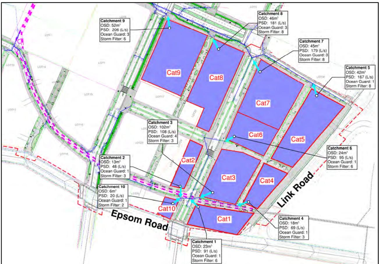
Figure 11 – Proposed Stormwater Concept Plan
